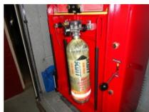
6. Open the charging chamber door lock by operating the handle on the right side of the chamber so that the yellow lock bars are **NOT** showing.
