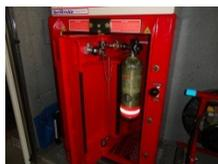
8. Close and lock the charging chamber door handle. The door is locked when the yellow lock bars are visible around the door frame.
