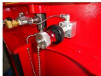
4. To charge two cylinders, remove the plug from the other charge adapter and mount the second cylinder. Hand-tighten the charge adapter.
