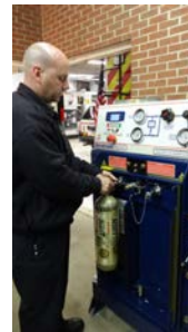
Attach SCBA Cylinder to Charge Adapter
