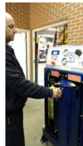
Rotate Chamber Door the cylinder is inside the fill station
