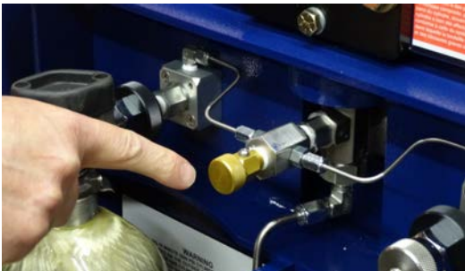
Open Bleeder to release pressure Then Close Bleeder
